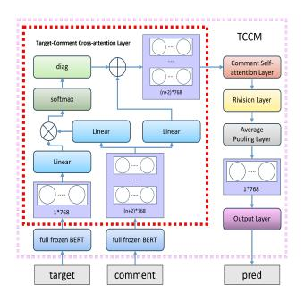
Figure 1: Structure of the TCCM
